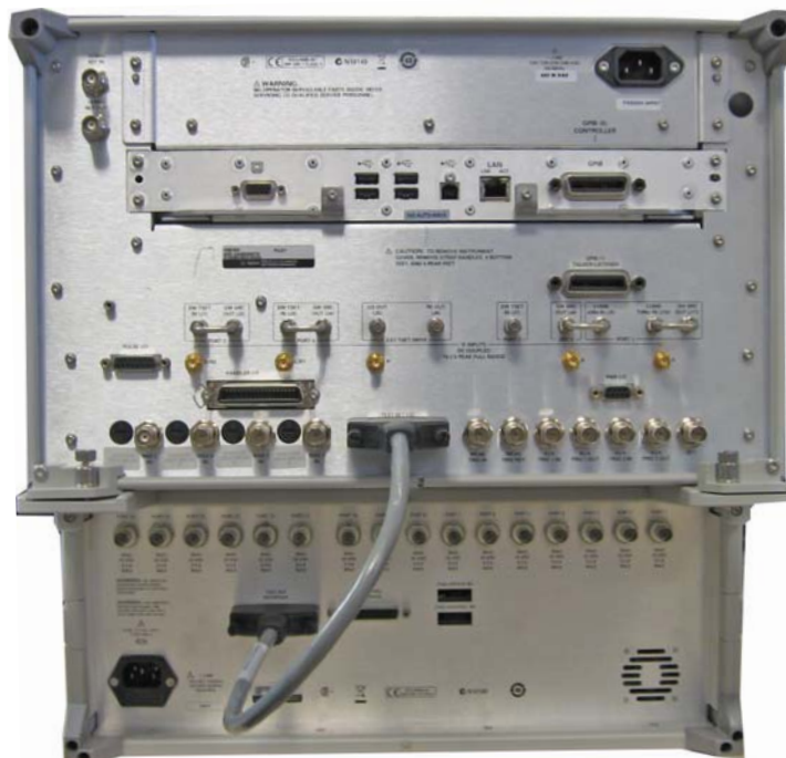
Figure 29 N5242A Test Set I/O Cable Connection
